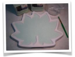
Fire the mold according to the Casting Schedule. The firing schedule's low target temperature and long hold will prevent the frit from becoming too liquid and balling up due to surface tension.
